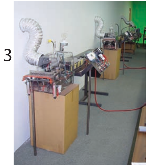
Each of our three electro-pneumatic fin molding machines can produce millions of parts per year. They heat, mold and cut out the finished pieces.
