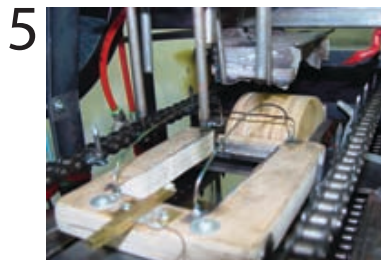
Closeup of the hotwire cutter, mold and cooling nozzles. The 2-part mold presses on both sides of the hot plastic to shape it. The hot wire melts through the plastic from below to cut out the finished piece.
