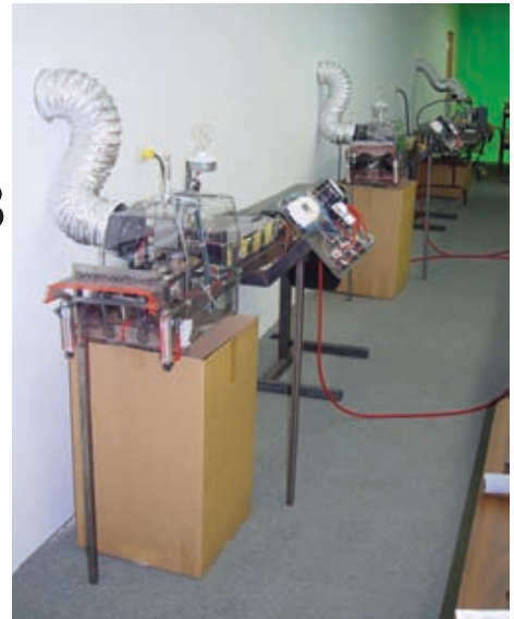
Each of our three electro-pneumatic fin molding machines can produce millions of parts per year. They heat, mold and cut out the finished pieces.
